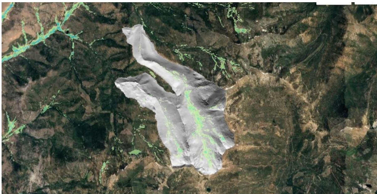
Figure 12. LiDAR analysis of Project catchments (Gray). Light green shading represents areas modeled to have a high potential to support meadow floodplain habitat while the darker green represents current meadow habitats.
