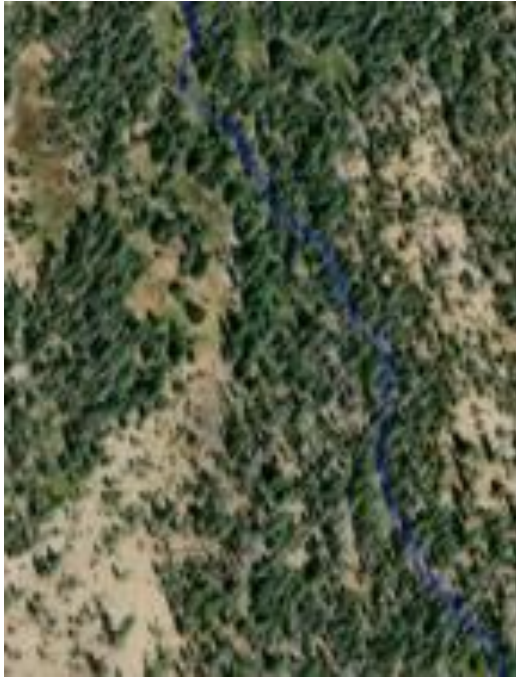
Figure 7: Step 1: Generate LiDAR derived flow path. This flow path near the top of the Cabin Meadow watershed appears to flow through a series of small meadow lobes and conifer forests. Nearby to the west there appears to be a dry meadow lobe
