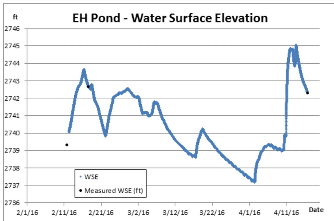
**Figure 17: Calculated and measured water surface elevation – EH Pond.**
