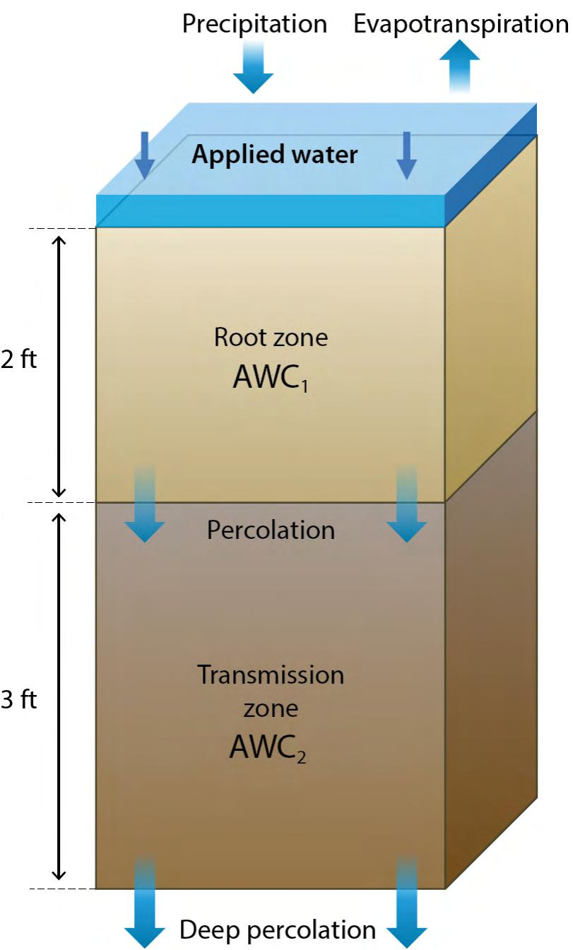
**Fig. 2.** Conceptual diagram of two-layered soil water balance model. The root zone is modeled with the Thornthwaite-Mather procedure and includes the loss of soil water by evapotranspiration. Saturated and unsaturated flow in the transmission zone is modeled with a one-dimensional vertical flow model receiving only the deep percolation from the root zone as water input. AWC is the soil-specific available water capacity. Variables are explained in the technical appendix.
