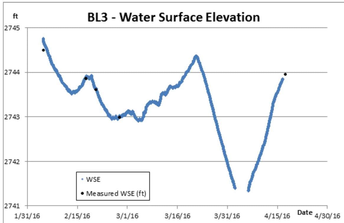
Figure 11: Calculated and measured water surface elevation –BL3.
