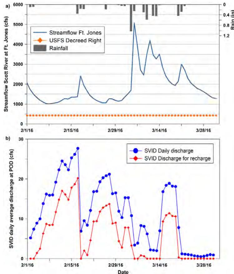
**Figure 1:** Daily average discharge (cfs) at USGS stream gauge near Fort Jones (USGS 11519500) (a) and at the SVID point of diversion (POD) (b). The orange dotted line in (a) indicates the minimum flow requirement of 426 cfs specified in the Scott River Decree.
