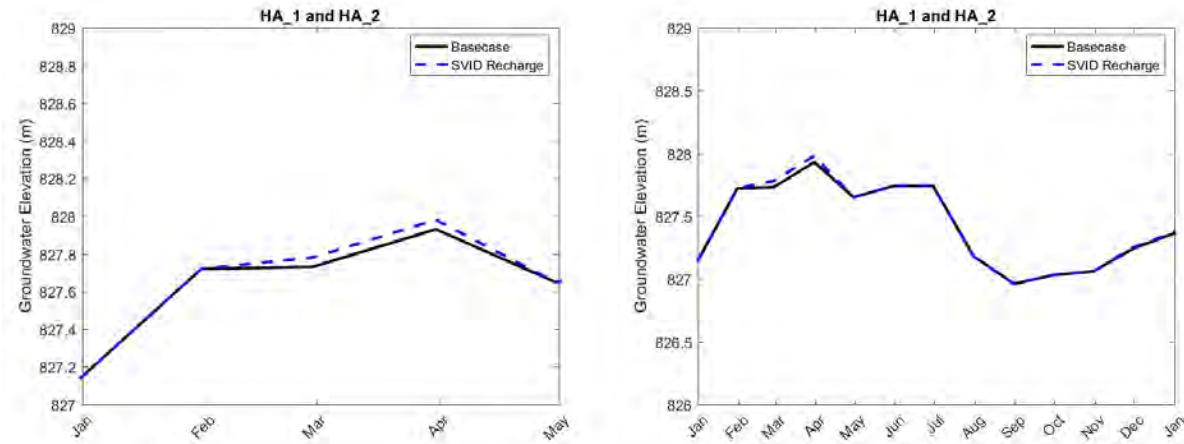
**Figure 29:** Modelled vs. observed groundwater elevation at locations HA1 and HA2 for Jan. 1 – May 1, 2016 (left) and the 2016 calendar year.
