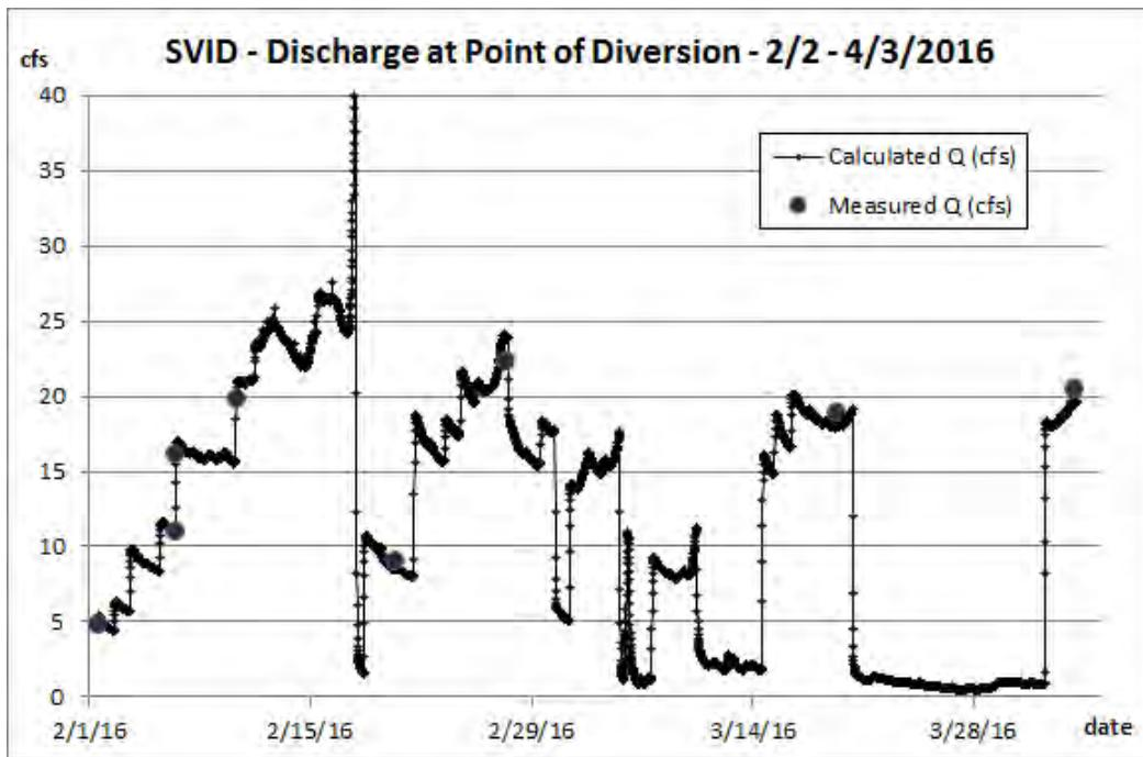
Figure 2: Calculated and measured discharge (cfs) at SVID point of diversion – 2/1 – 4/3/2016.
