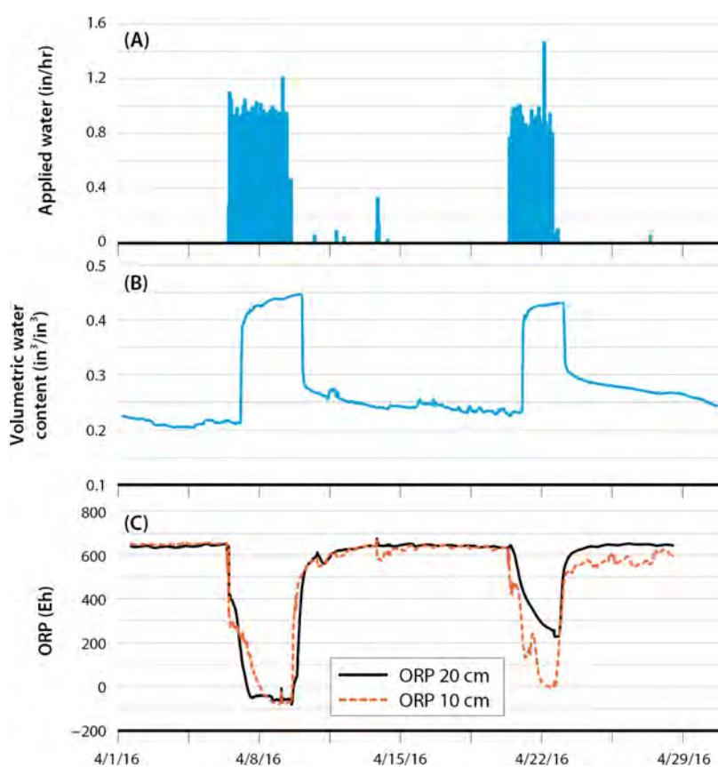
**Fig. 7.** Precipitation and applied water (A), volumetric water content at 8 in depth (B) and oxidation-reduction potential measured at 10 am (red dots) and 20 cm depth (black line) (C) at the Scott Valley site.
