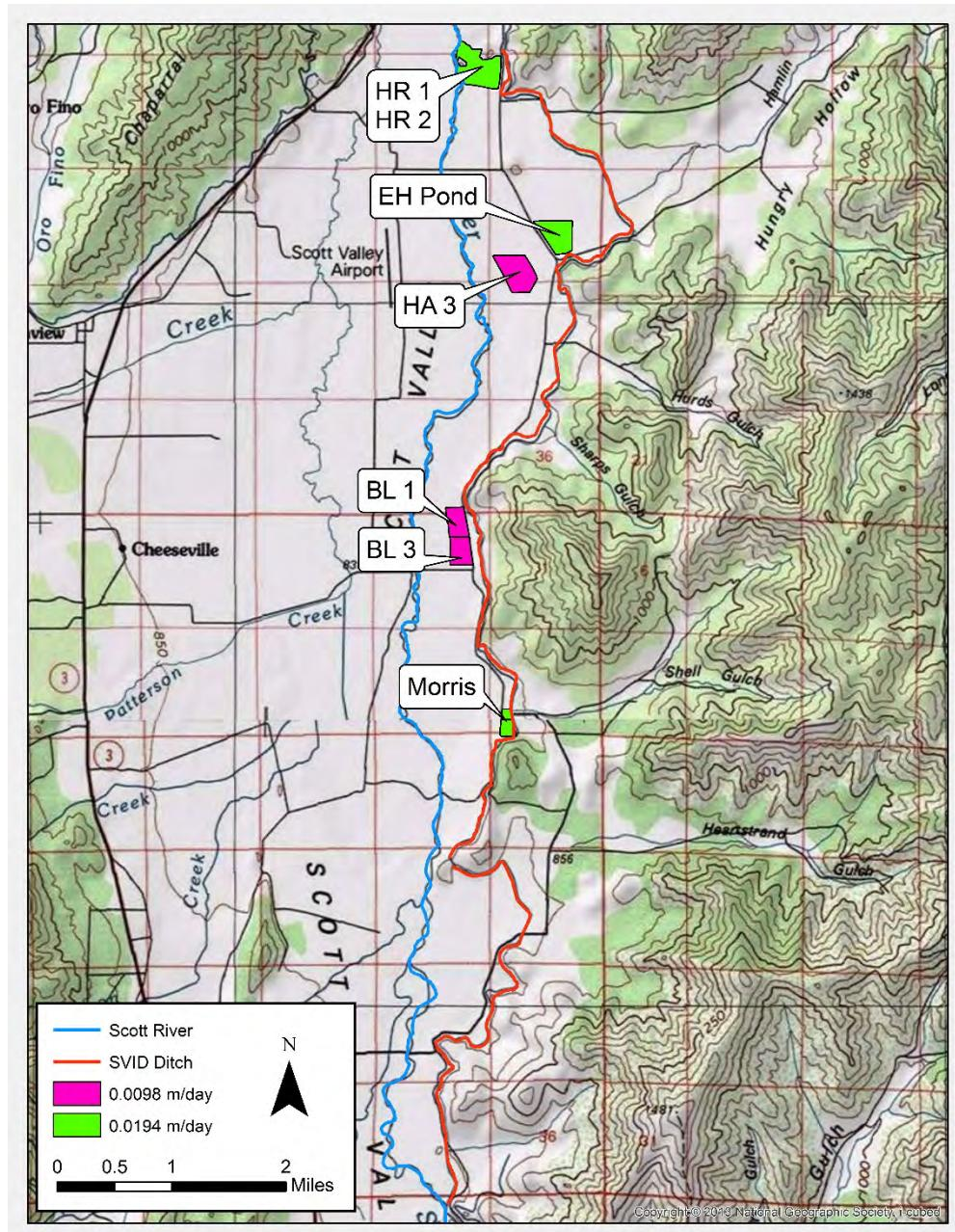
**Figure 25: Recharge locations and recharge rates from on-farm flooding assumed in the SVIHM model.**
