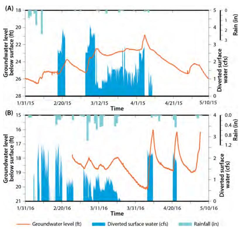
**Fig. 5.** Amount of winter water applied for recharge (cfs), change in depth to the groundwater table (ft) and rainfall (in per day) measured between January and May in 2015 (A) and 2016 (B) for the Scott Valley site.
