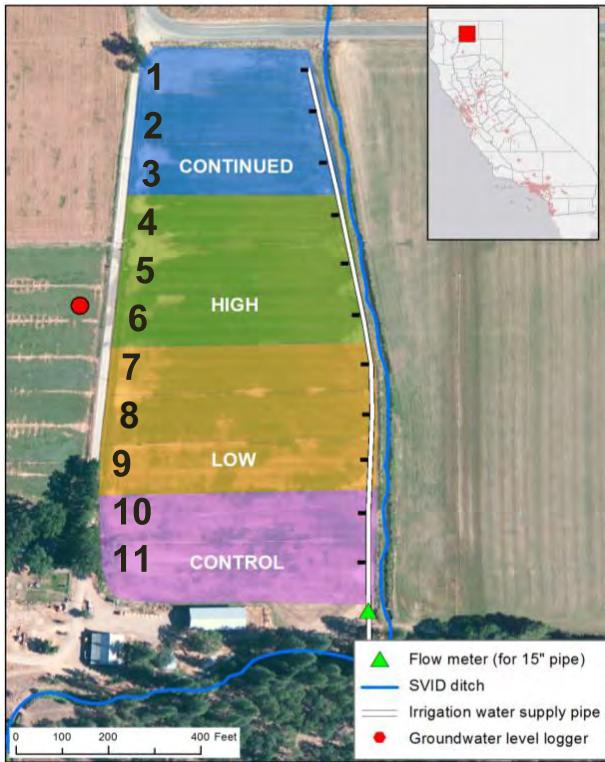
**Figure 33: 15-acre field with 10-year alfalfa stand. Three different water application rates were tested: continued, high, low and no water (control) application. Numbers indicate individual checks.**
