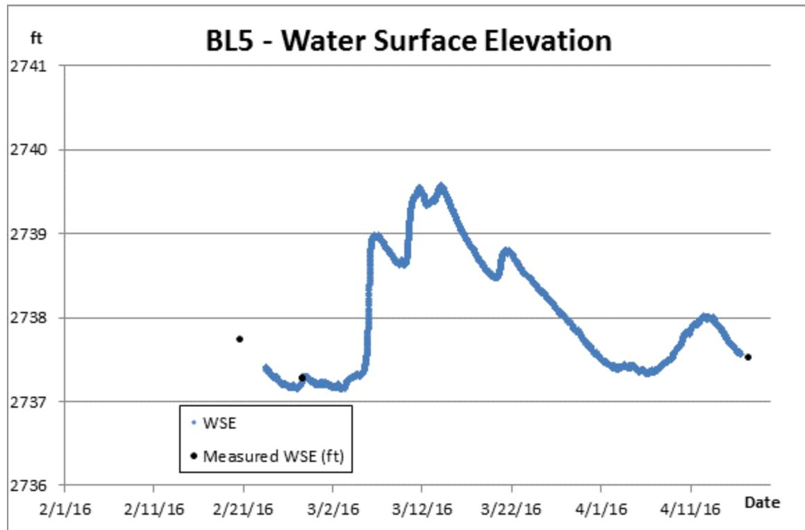
**Figure 15:** Calculated and measured water surface elevation – BL5.
