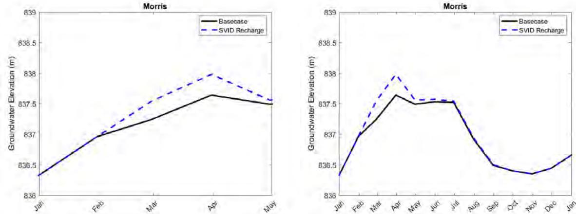
**Figure 31:** Modelled vs. observed groundwater elevation at location JM1 for Jan. 1 – May 1, 2016 (left) and the 2016 calendar year.
