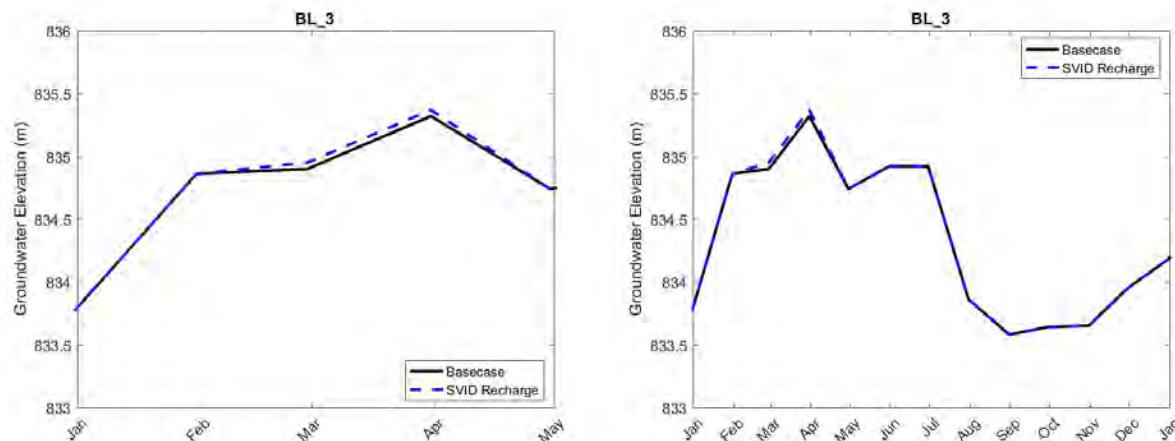
**Figure 27:** Modelled vs. observed groundwater elevation at location BL3 for Jan. 1 – May 1, 2016 (left) and the 2016 calendar year.
