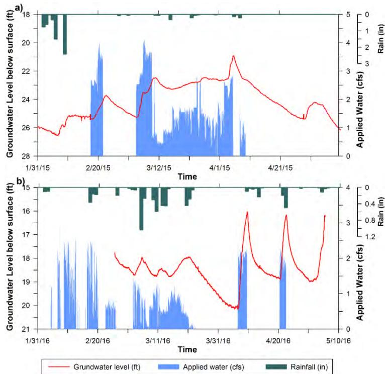
**Figure 34: Amount of water diverted for winter recharge (cfs), change in groundwater level below surface (ft) and rainfall (in) measured in winter 2014/15 and 2015/16.**
