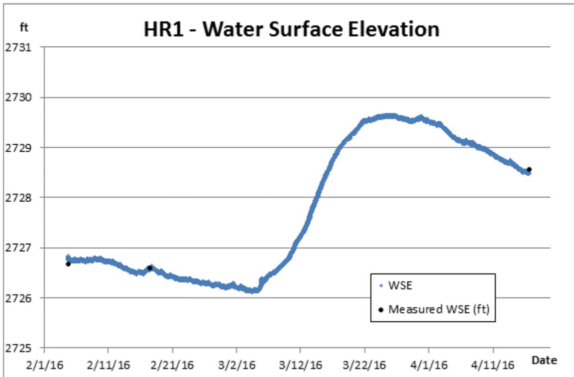
Figure 21: Calculated and measured water surface elevation – HR1.
