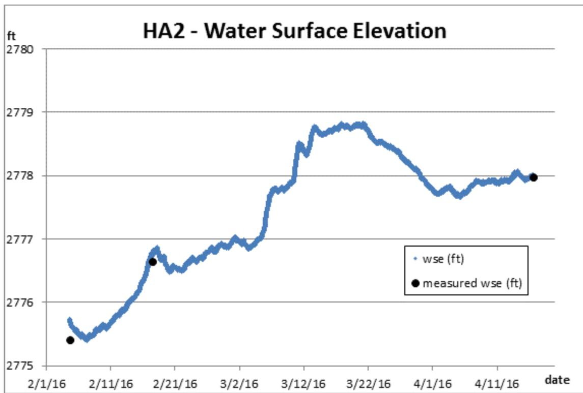
Figure 7: Calculated and measured water surface elevation – HA2.
