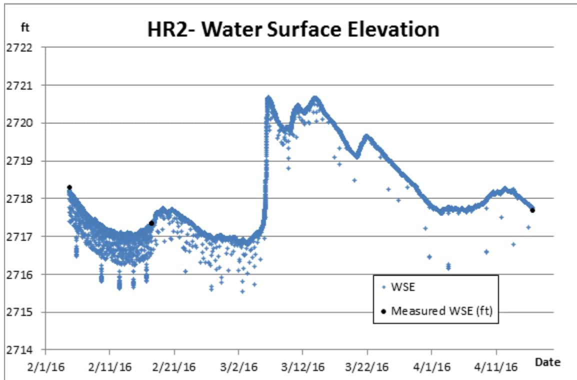
Figure 23: Calculated and measured water surface elevation – HR2.
