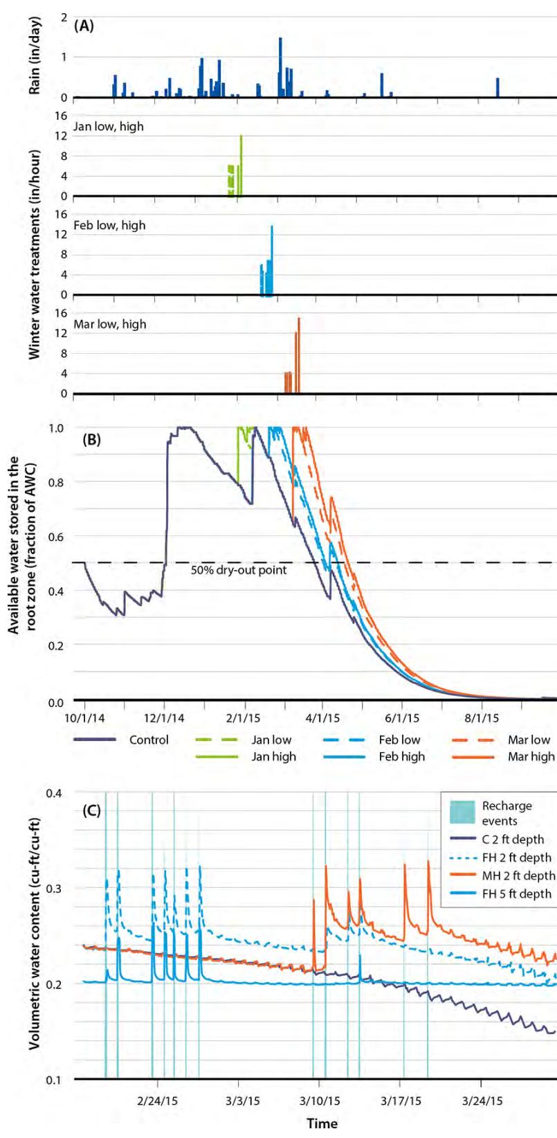
**Fig 3. Water balance summary for the Davis site. (A) Daily precipitation and timing of winter water treatments. (B) Change in available soil water in the root zone (0–2 ft) as fraction of the soil-specific available water capacity (AWC). (C) Measured change in soil water content at 2 ft and 5 ft depth. Deep percolation occurred when volumetric soil water content was at a maximum.**
