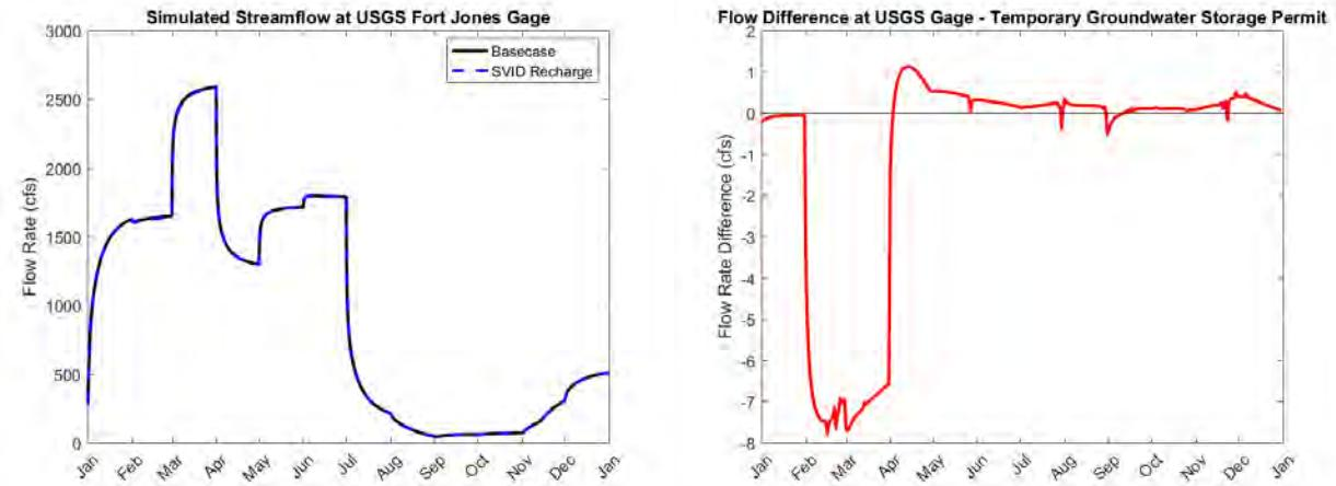
**Figure 32:** Comparison of simulated streamflow at USGS Fort Jones stream gauge between the base scenario (black line) and the recharge scenario (blue line) (left) and flow difference for the 2016 calendar year (right).
