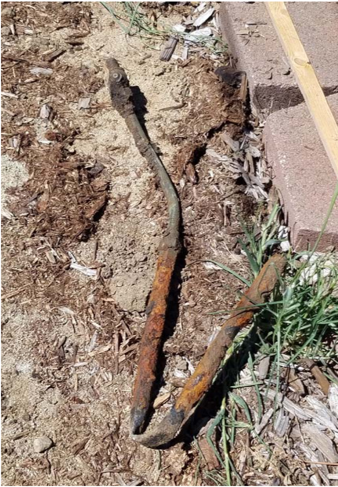
Photo 1 - Old service line and corp stop pulled from existing 4-inch AC pipe during the Third Ave. Main Replacement Project.
