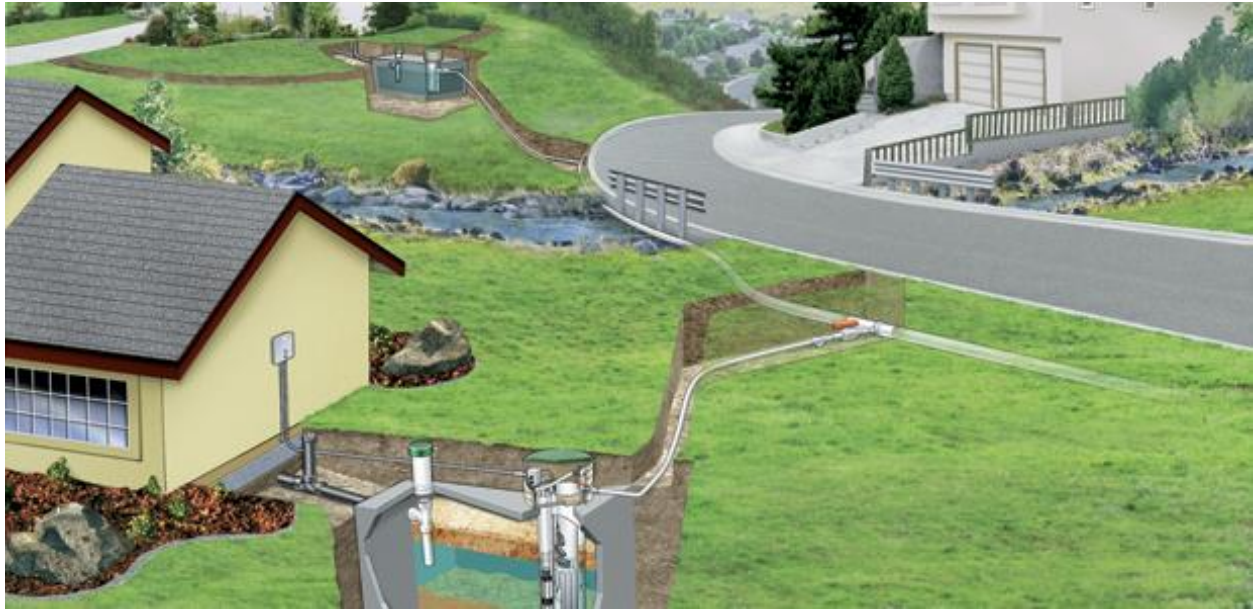
Figure 1: Typical Residential Setup to a Cluster System (Photo credit: Credit South Blount County Utility District)
