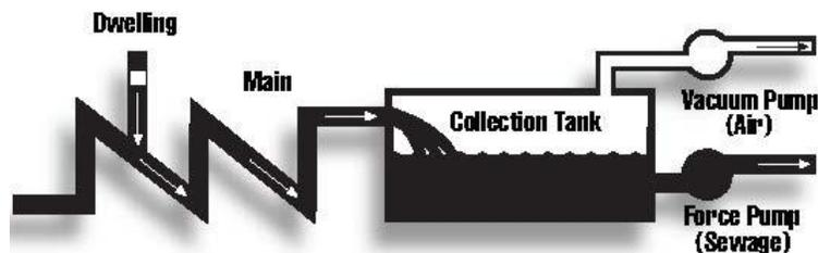
The pipe is designed to follow the contour of the land where the ground slopes naturally, and is most economical in flat terrain. Small lifts in the pipe may be used when necessary to keep excavation shallow. At the pumping station, the mains empty into a collection tank. The wastewater is then treated nearby or pumped to another location for treatment.
