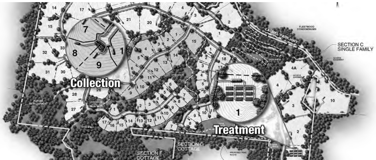
Figure 1. Orenco STEP System and AdvanTex Treatment Facility
