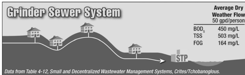
Figure 16. Grinder sewer system profile (typ.)
